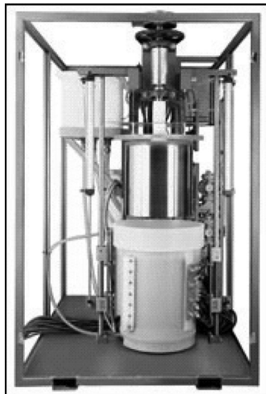
FIGURE 9.15 An electrowinning system using a rotating electrode to improve metal yields and allow economic metals recovery from solutions with lower metals concentrations.
